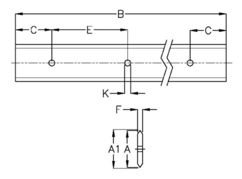
$\begin{array}{lll} A & = 76 \\ A1 & = 76.81 \\ B & = 3416 \\ C & = 43.0 \\ E & = 90 \\ F & = 9.12 \\ For bearing = J54 \end{array}$
